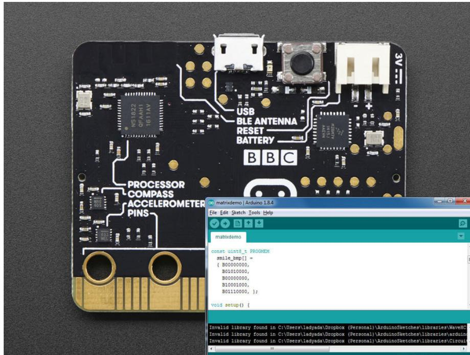
Did you know that the Arduino IDE can be used to program the micro:bit? Now you have yet another way to use this cool board! Learn how to set up Arduino to program your micro:bit, blink some LEDs, read the internal temperature sensor, send and receive data over Bluetooth - even log data to Adafruit.IO!
