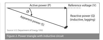
when voltage is applied, which produces a slight delay in the current. Because of this phenomenon, we can say that for an inductive circuit, current lags the voltage, and the circuit has a lagging power factor (Blume 2007; U.S. Department of Energy 1992). A diagram of the active, reactive, and apparent power components in an inductive circuit is shown graphically in Figure 2.
