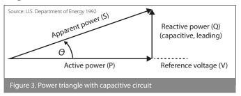
Typical distribution circuits contain resistive and inductive loads; therefore, utilities install capacitors to balance the var requirement (Blume 2007).
