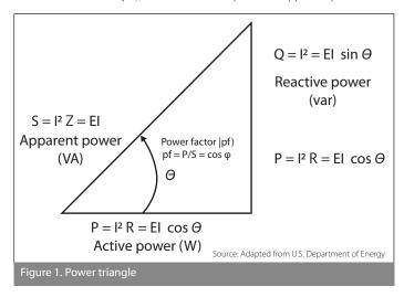
The equations for calculating these values from basic electrical quantities of root mean square voltage (E), resistance (R), reactance (X), impedance (Z), and root mean square current (I) are also shown in Figure 1.
