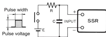
The value of R and C must be decided carefully. The value of R must not be too large or the supply voltage (E) will not be able to satisfy the required input voltage value. The larger the value of C is, the longer the release time will be, due to the time required for C to discharge electricity.
