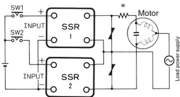
Note 1. The voltage between the load terminals of either SSR 1 or SSR 2 when turned OFF is approximately twice as high as the supply voltage due to LC coupling. Be sure to use an SSR model with a rated output voltage of at least twice the supply voltage. For example, if the motor operates at a supply voltage of 100 VAC, the SSR must have an output voltage of 200 VAC or higher.
