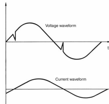
An inductance (L) load causes a current phase delay as shown on the left. Therefore, the loss is not as great as that caused by a resistive (R) load. This is because a high voltage is already imposed on the SSR when the input current to the SSR drops to zero and the SSR is turned OFF.
