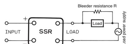
Bleeder resistance standards: 100-VAC power supply, 5 to 10 kΩ, 3 W
