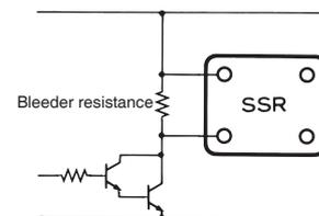
The bleeder resistance R can be obtained in the way shown below.
