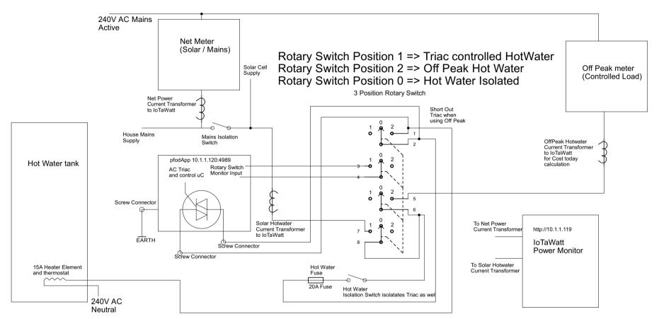
Solar Cell Hot Water (c)2023 Forward Computing and Control Pty. Ltd. NSW. Australia, www.forward.com.au
